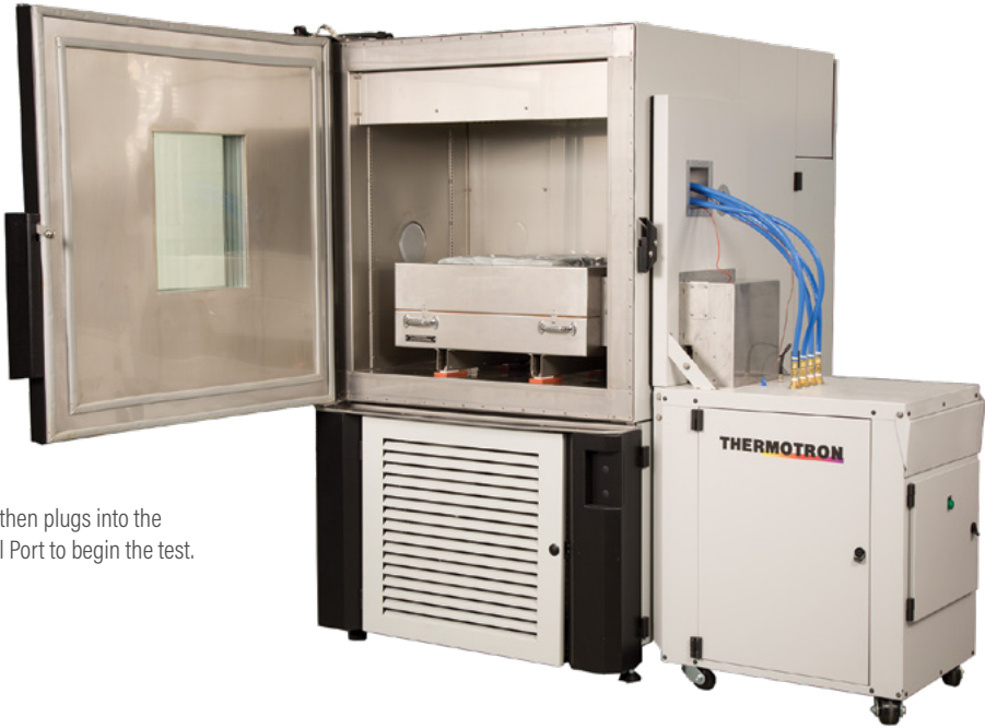
Step 1: The cart stores the shaker when not in use and allows the chamber to be used on its own.
