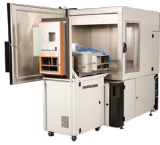
Step 2: The integrated loading ramp and shaker casters simplify shaker-to-chamber transition.
